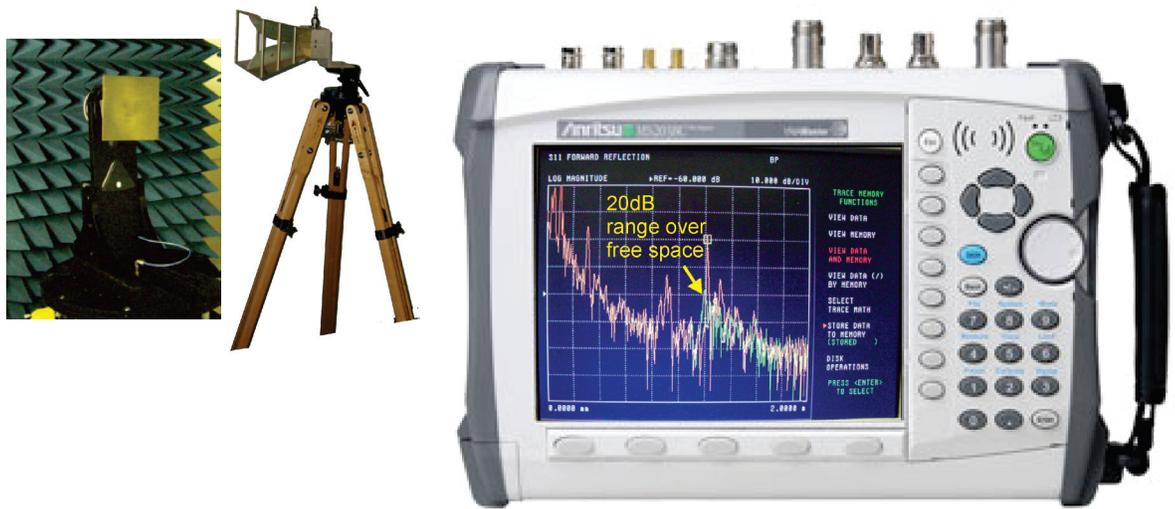
Set the measurement distance to 1.25m with a 6" range and apply the time gate so that only the plate reflection is seen.
