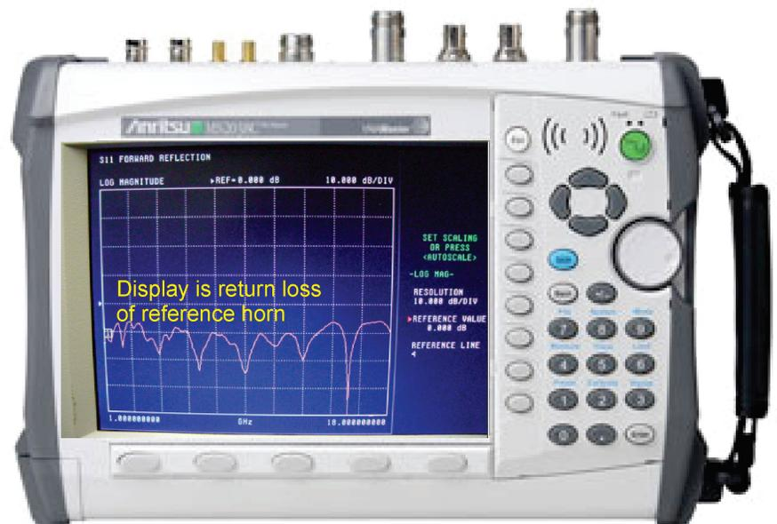
Initiate time domain and distance. Notice the S11 drops to below -50dB at distance compared to the -10dB at near 0m(the horn reflection). With the plate reference at right angle (Use DAMs jog) store the trace into memory and display data and memory. The rotate the plate to full reflection and observe the position with the marker(1.25m) set to the peak change.
