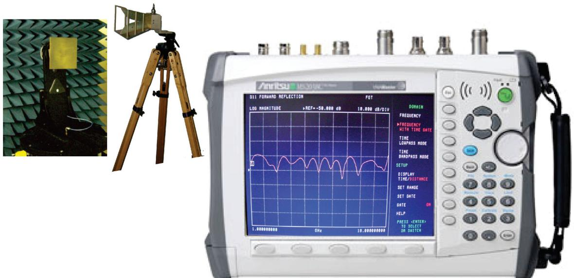
With the DAMs Azimuth set to 0-360 with 10 degree steps, load the RCS measurement schematic and invoke the FSM RCS measurement/calculation. Minus (-) is de-embed.
